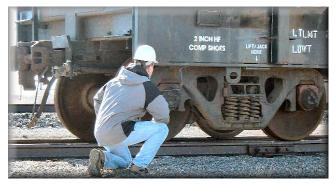
inspect welds that are not readily accessible. All NDT inspections of welds start with visual inspection. This is purposely done and sometimes is required by the NDT procedure so visible discontinuities can be addressed prior to subsequent NDT being completed.
