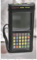
discontinuities. If an anomaly is found, the sound energy is returned to the transducer and a signal is displayed that provides the location of the discontinuity in the weld or component. This method requires a higher skill level and more training than other NDT methods. Access is only required from one side of the object.
