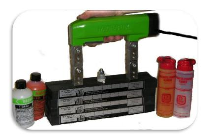
Since magnetic properties are involved, MT is limited to ferrous (iron) based materials.
