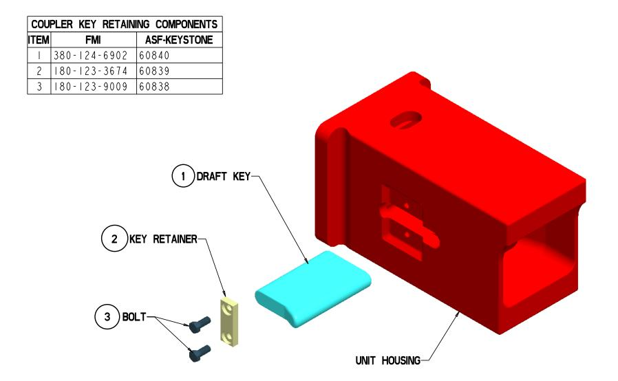
INSTALL COUPLER, DRAFT KEY, KEY RETAINER AND BOLTS, TORQUE TO 20-35 FT/LBS RETAIN EACH BOLT BY TACK WELDING THE BOLT HEADS TO THE KEY RETAINER
