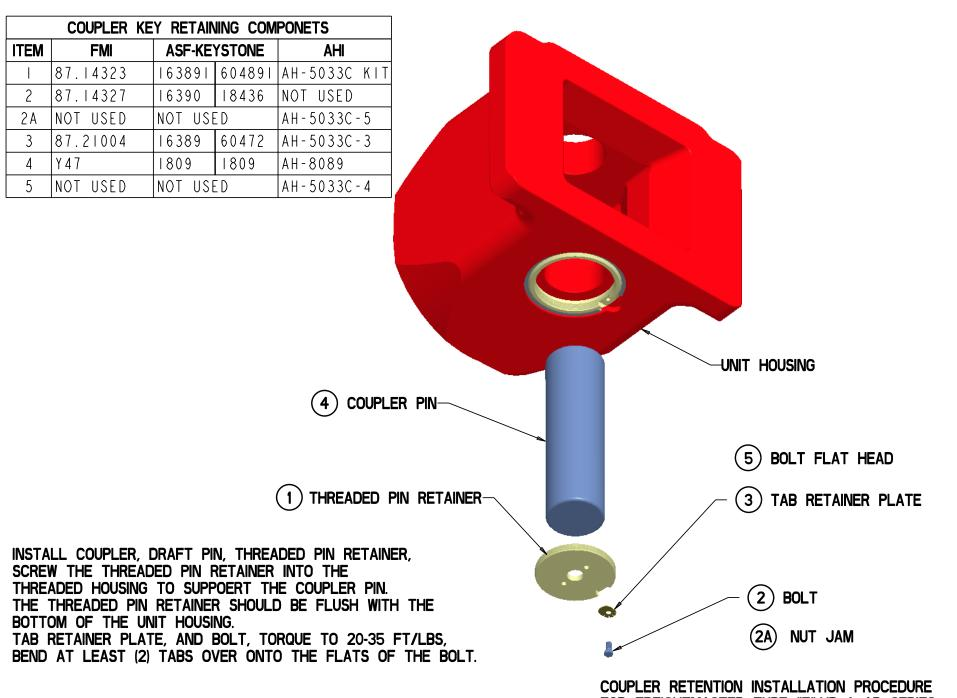
COUPLER RETENTION INSTALLATION PROCEDURE FOR FREIGHTMASTER TYPE "F"-HD & AR SERIES STYLE APPLICATION
