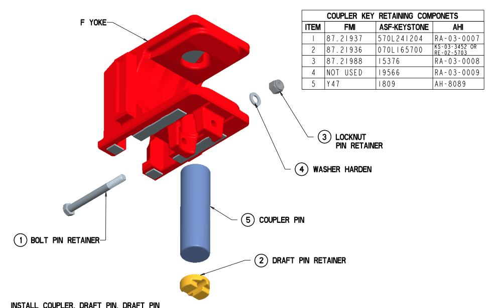
INSTALL COUPLER, DRAFT PIN, DRAFT PIN
